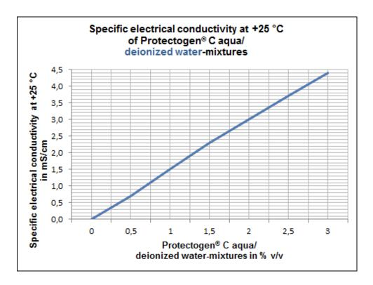
In case that no deionized or distilled but tap- or drinking water will be inhibited with Protectogen<sup>®</sup> C aqua, the final concentration can be determined as follows:
